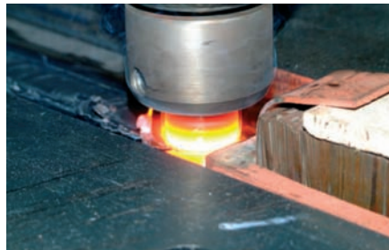
Friction stir welding of high strength structural steel with inductive preheating process
